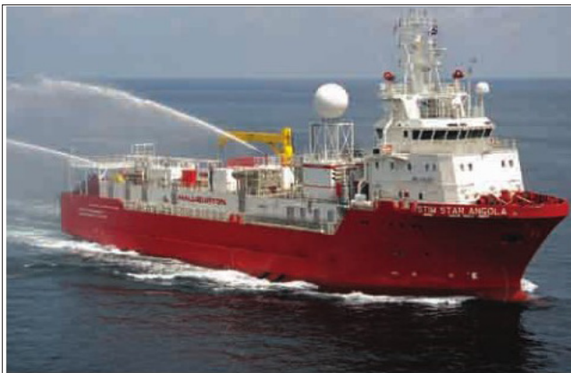
Fig. 2 —Equipped with 8,250 hhp and 15,000 psi-capable pumps and manifolds, Halliburton's Stim Star Angola delivers a wide range of stimulation services offshore West Africa. Photo courtesy: Halliburton.
